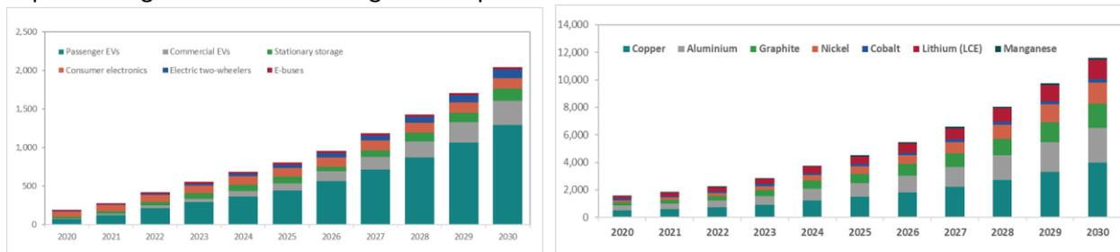
Figure 26 LHS: Annual Li-ion battery demand in GWh; RHS: Metals demand from all Li-ion batteries (thousand metric tons)<sup>53</sup>
