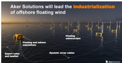
Figure 9 Ecosystem of offshore floating and example provided by Aker Solutions<sup>24</sup>
