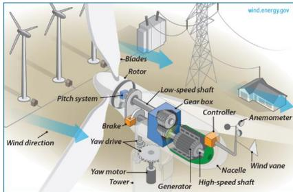
Figure 8 Inside of a wind turbine and ecosystem of onshore wind<sup>23</sup>
