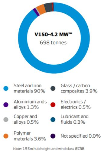
Figure 11 Materials required in a Vestas V150 4.2MW turbine<sup>26</sup>
